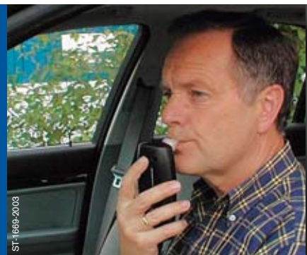
Figure 2: Submitting a breath sample to an interlock
