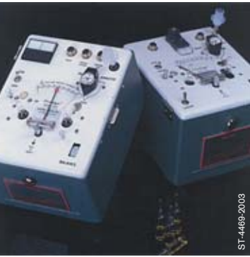
Figure 6: Dräger Breathalyzer using wet chemical analysis procedure
