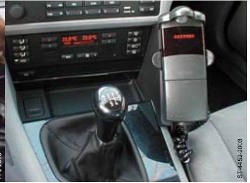
Bild 12: The Dräger Interlock, an alcohol ignition interlock device, in the year 1995
