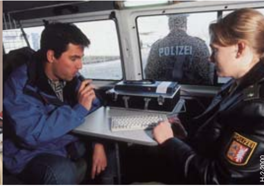
Bild 11: Alcotest 7110 Evidential with infrared optical and electrochemical sensor in the year 1998
