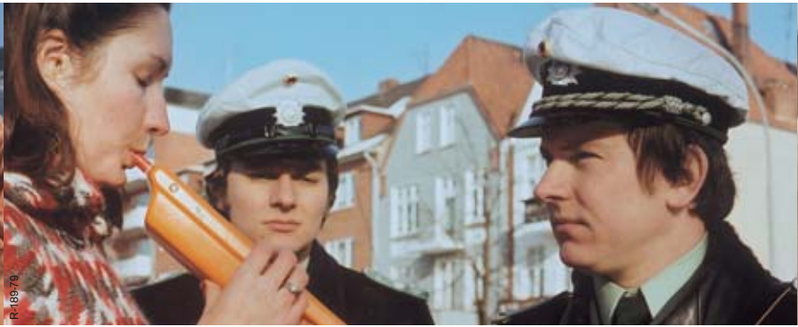
Figure 9: The Alcytron prototype with an infrared optical sensor in the year 1978
